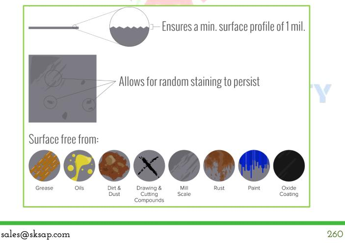
This standard governs surface preparation for non-ferrous metals before the application of a protective coating. It is used when adding a surface profile to stainless steel, galvanized steel, copper, and other metals that are not carbon steel. It requires a minimum surface profile of .75 mil 19 micrometers) and for the surface to be free of loose coating and other contaminants, as verified by a visual inspection.
