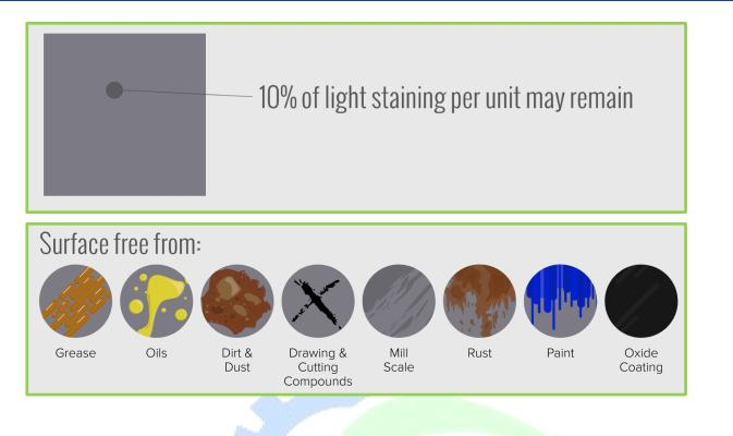
II. SSPC-SP15- Commercial Grade Power Tool Cleaning Like SP11, this standard describes the requirements for taking a surface to bare metal, while ensuring a minimum surface profile of 1 mil 25 micrometers). Unlike SP11, SP15 allows for random staining to persist on the substrate.
