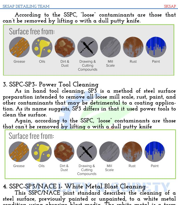
condition using abrasive blast media. The white metal is a term used to describe a surface that's uniformly free of all foreign matter and white or gray in appearance.
